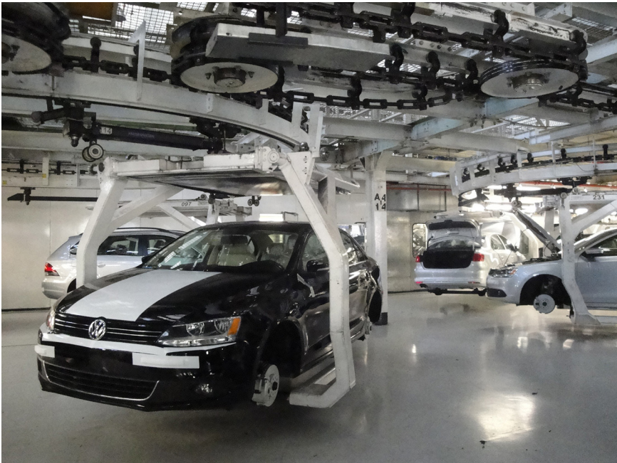
Figure 1. Almost-finished cars moving on the assembly line. Photo by Alejandra González Jiménez.
