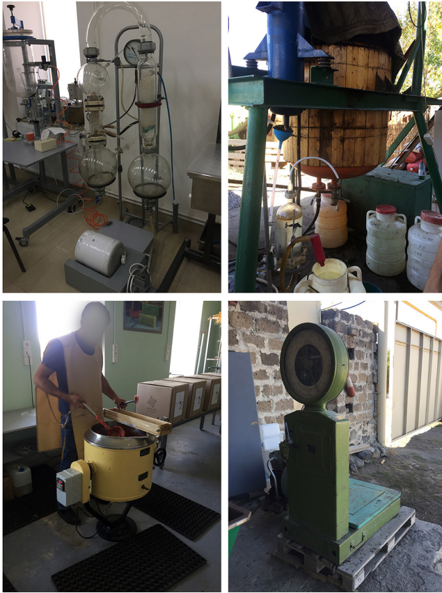
Figure 6. Refitted and upcycled equipment from Khimzavod at the Nairian factory: distillery from old flasks (top left); distillery from old autoclave (top right); cauldron used for saponification (bottom left); Soviet vintage scale to weigh plants (bottom right). Photos by Lori Khatchadourian.
