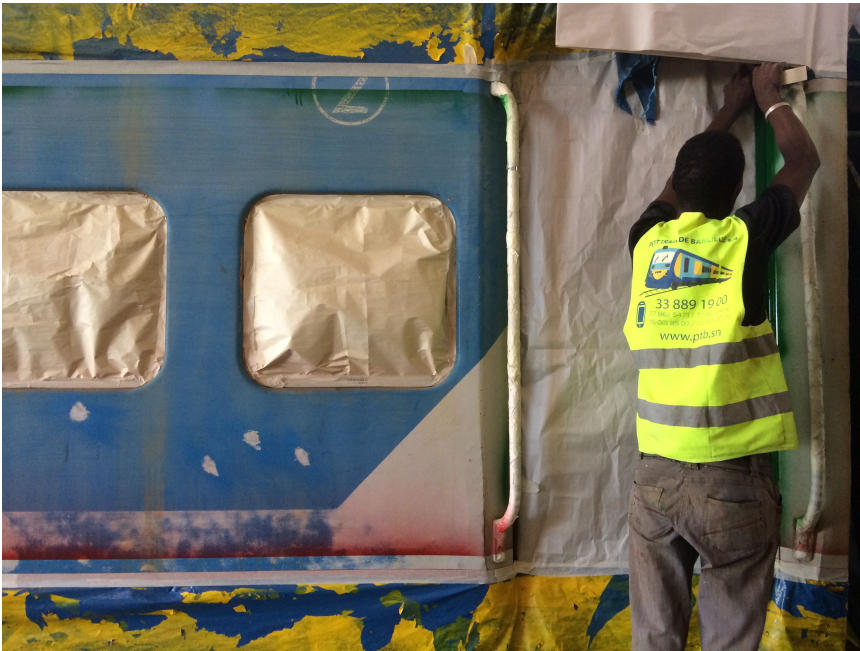
Figure 15. Preparing a carriage in Rufisque for repainting—a form of cosmetic repair that restores appearance more than function. Photo by Charline Kopf.
